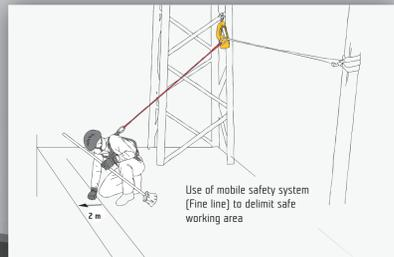
Use of mobile safety system (Fine line) to delimitate safe working area.
